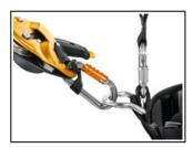
The Am'D carabiner has an asymmetric D shape that is ideal for attaching equipment such as descenders or positioning lanyards. Usage of the CAPTIV positioning bar favors loading of the carabiner along the major axis, limits flipping and keeps it attached to the device or lanyard.
