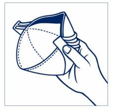
1. The noseclip is located in the top panel. Pre-form the noseclip by gently bending at the centre of the panel. Hold the respirator in one hand and pull out the bottom panel to form a cup.
