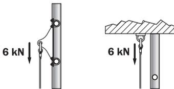
For all other configurations, the anchorage should support a load of 6kN minimum in the direction of the cable. If necessary, contact Tractel SAS.
