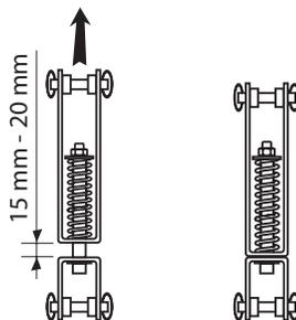
COMMENT: Adjustment between 15 and 20mm corresponds to a maximum load under tension of the lifeline of 50 daN.
