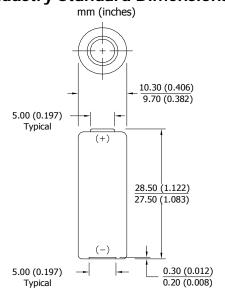
Designed for electronic applications which may require high rate pulses. Classification: Miniature Alkaline
